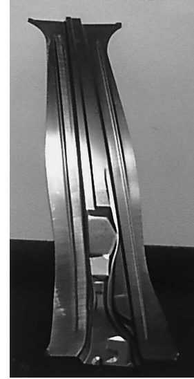
Photo 7 Applied example for center pillar reinforcement of TS980 MPa steel sheet (low YR type) (Formed by the experimental stamping tools in JFE Steel)
